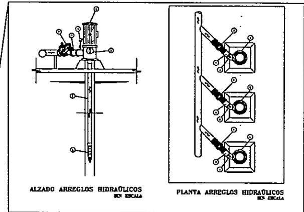
ALZADO ARREGLOS HIDRAULICOS EN ESCALA
